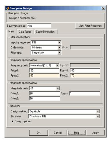
**3** Enter the correct frequencies for **Fpass2** and **Fstop2**, as shown in the preceding figure, then click **OK**. Here the specification uses normalized frequency, so that the passband and stopband edges are expressed as a fraction of the Nyquist frequency (in this case, 48/2 kHz). The following message appears at the MATLAB<sup>TM</sup> prompt:
